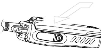
Then firmly press the battery pack downwards to lock it in place until a click is heard.
