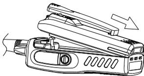
Match the 3 bulges of the battery pack with the corresponding slots at the rear bottom of the transceiver.
