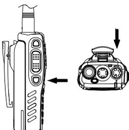
Press the button preset as canceling squelch to listen to the background noise and rotate the Power/Volume switch to adjust capacity.
