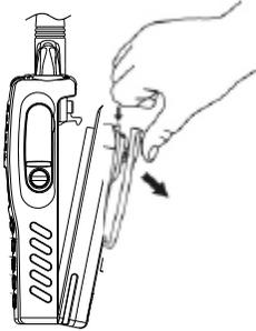
To remove the battery pack, use your thumb to press the belt clip, one side of your index finger to press the release button and then pull the battery away from the radio
