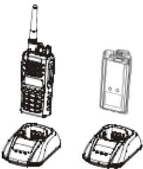
Insert the battery or transceiver into the charger slot, and make sure the transceiver has been turned off.
