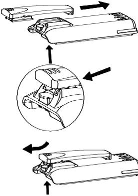
Match the grooves of the belt clip with those on the rear of the battery. Then press belt clip downwards to lock it in place. Push the card by inserting your nail or tool into the groove at the upper part of the clip to remove the belt clip.
