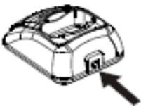
Plug the power adapter into the proper AC wall outlet; and then the green indicator lights.
