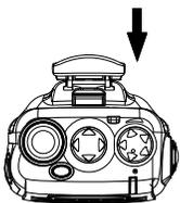
Switch on the radio by turning the Power/Volume switch clockwise till a click is heard, then the radio will be in the state of stand by and you will hear a beep if the dealer has set it.
