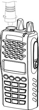
Screw the antenna into the connector at the top of the transceiver by holding the Button of the antenna and turn it clockwise until secure.
