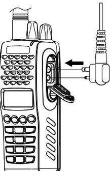
Insert the speaker/microphone plug into the jacks of the versatile connector, and fix it with the supplied snail screw.
